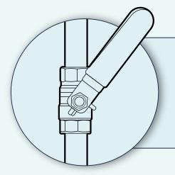
Example of a typical internal shut off valve, although the appearance may vary slightly. If this shut off valve turns all the fresh cold water off inside your home you have located your internal main water supply line.
